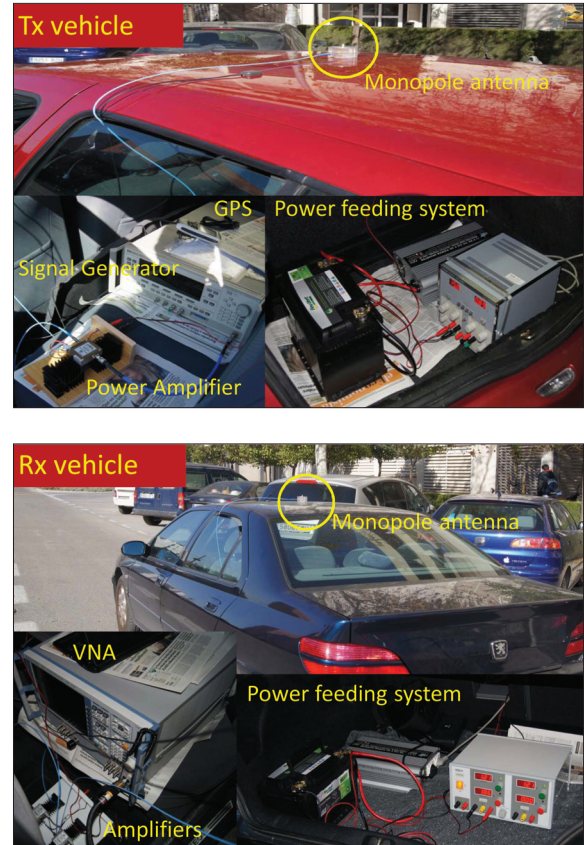
■ Figure 3. On board system setup: (a) Tx vehicle and (b) Rx vehicle.
