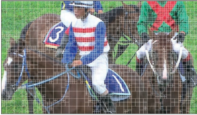
■ Figure 5. Picture partitioning into Coding Tree Blocks.
