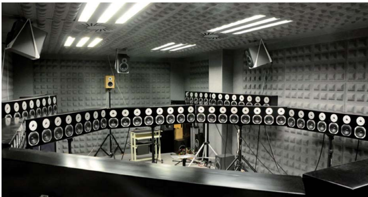
■ Figure 4. Wave-Field Synthesis set-up, where the octagon with the 64 loudspeakers can be appreciated and also the reference loudspeakers at the back in brown color.
